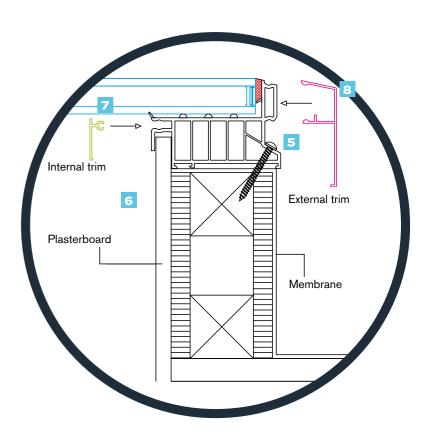
Before lifting the glazed rooflight onto the kerb structure, run a silicone seal on top of the kerb membrane.
